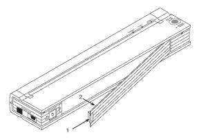
Figure 10. Opening the Battery Cover
